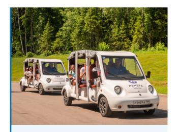
RENERA supplied six electric sightseeing cars equipped with Li-ion traction batteries to a theme park in Moscow regoin. The 26 KWh Li-ion battery produced by RENERA enables a maximum travel range of 100 kilometers. The battery can be charged using a standard 220V outlet. The charging process takes 6 to 10 hours. Since electric vehicles produce no emissions and run almost noiselessly, tourists can enjoy the signing of birds and rustling of leaves in the park.
