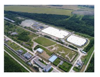
According to Andrey Lebedev, Director for Environmental Programs at Rosatom, a waste treatment plant was piloted at a hazardous waste landfill site near Krasny Bor, Leningrad Region. After a multi-stage treatment, liquid wastes are turned into a dry geocomposite material and water, which is clean enough to be used in fish ponds. Tests conducted by an independent laboratory show that the waste treatment plant does its job well.
