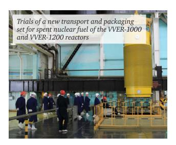
It also processes spent fuel without creating liquid waste. Isotope Chemical Factory, a subsidiary of MCP, manufactured nuclear casks, flasks, ampoules and other equipment for spent nuclear fuel management and provided transportation and storage services for RBMK-1000 and VVER-1000 spent fuel. The factory operates wet and dry storage facilities.
